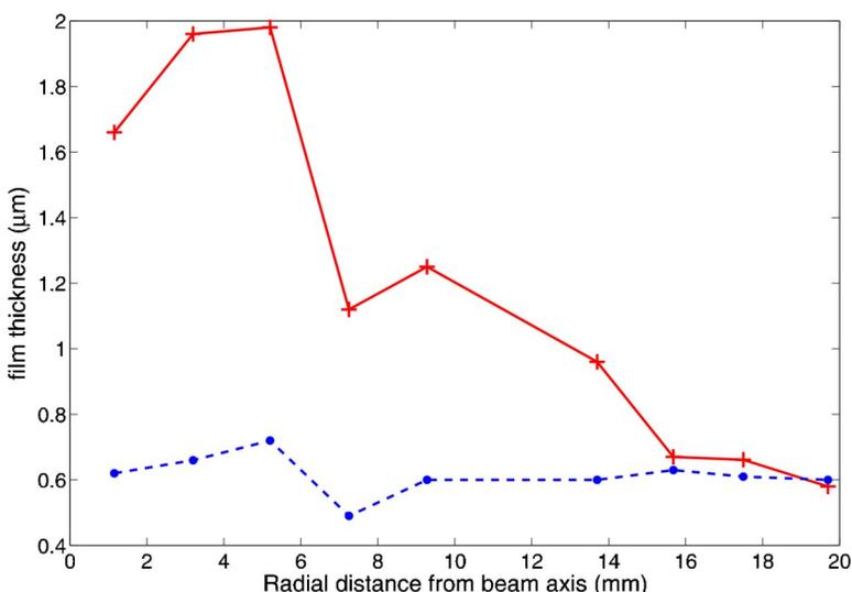
FIG. 2. (Color online) Radial thickness profile of a nanostructured  $\text{TiO}_2$  film by atomic force microscopy (AFM) with and without a graded exposure screen for the compensation of radial intensity variation.
