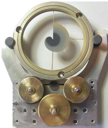
FIG. 3. (Color online) Graded exposure screen holder and rotator with screen mounted.
