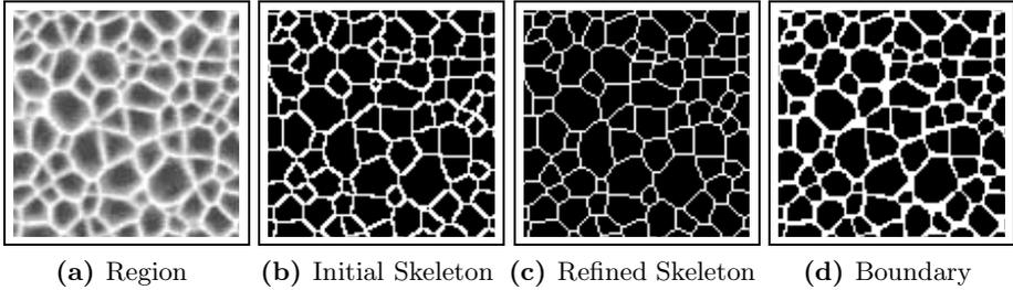
**Fig. 3.** Pore Segmentation steps: (a) locally processed region has (b) initial skeleton which leads to (c) refined skeleton used to find *local intensity threshold* yielding (d) boundary. Finally, the pores are defined as connected components separated by this boundary, as in Figure 2d.
