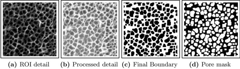
**Fig. 2.** Pore shape localization: A detail from the middle of an ROI is shown in (a). The ROI is locally equalized and re-quantized based (b), the pore boundaries are found (c) and finally a mask geometrically identifying all individual pores is created (d).
